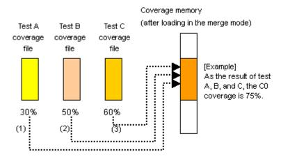
Figure 5.101 Schematic of merge mode applications
